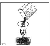
**3.** Using the funnel provided, pour in the salt until the container is full.
